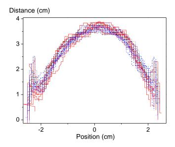
**Figure 5**: (color online) Successive shapes of the front during pulse displacement in the sample for the test shown in Figure 2: first upwards motion (red continuous), downward motion (blue dashed), second upward motion (black dotted).
