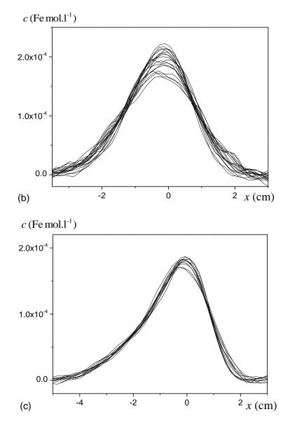
**Figure 7:** Shifted (see text) concentration profiles for different tests with close Peclet number values: (a) large beads with Pe = 447 (measured  $D/D_m = 210$ ); large beads with Pe = 431 (measured  $D/D_m = 148$ ); small beads with Pe = 426 (measured  $D/D_m = 63$ ). The volume fraction of particles is equal to *c* times 0.947 l.Fe mol<sup>-1</sup>.
