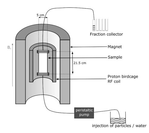
Figure 1: Scheme of principle of the experiment.
